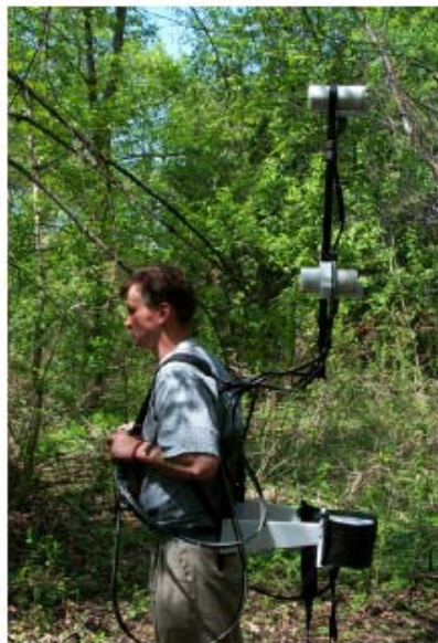
Figure 7: GEM GSM-19W Magnetometer system, configured with 2 sensors for gradient measurements (Ref [28]).
