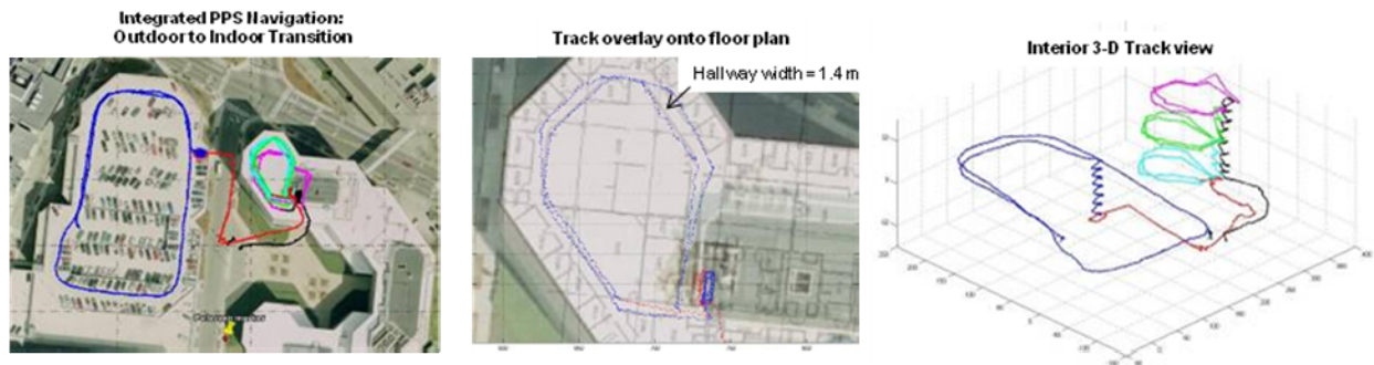
Figure 34: Indoor Navigation with Integrated PPS (Ref. [27]).
